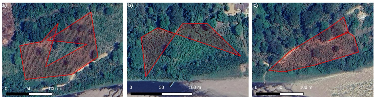
Figure 5. Examples of invalid polygon geometries. a) Self-intersecting polygon; b) Polygon with crossing boundaries; c) Polygon with an unclosed or improperly connected boundary segment.
